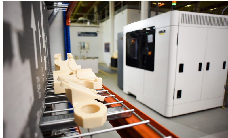
3D printed tooling produced on one of GKN Aerospace's 3D printers.
