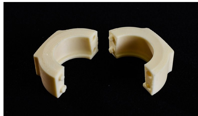
This small tool enables GKN to quickly cut new masks to the correct size and enables several parts to be processed at once.
